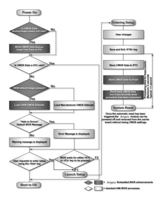
The above diagram provides an overview of how the BIOS Setup Data is backed up on modules. OEM default values mentioned above refer to customer specific CMOS settings created using the System Utility tool.
